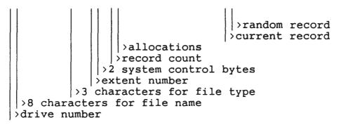
The first byte of a 36 byte FCB is the drive code. Here 1 means drive A, 2 means drive B, and so on. 0 signifies the default drive which simply means the drive that you are currently logged into.
